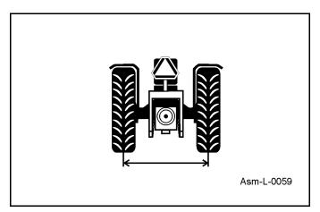
Add rear wheel weight, rear ballast box or implement. Make sure there is 20% of total weight on rear axle.
